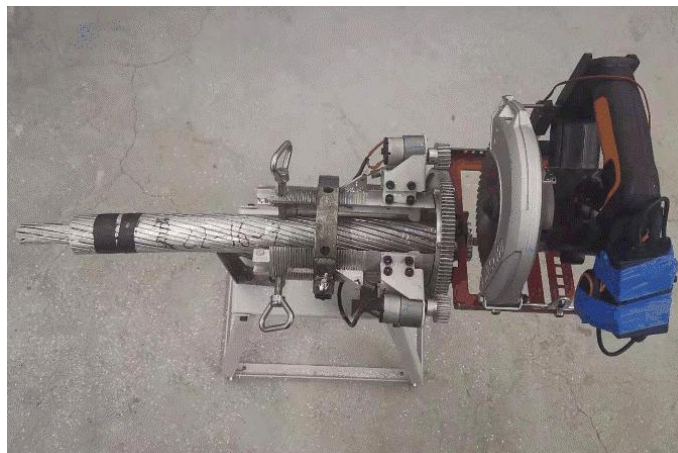
Fig. 4. Test device for multi wire diameter high voltage cable cutting machine
