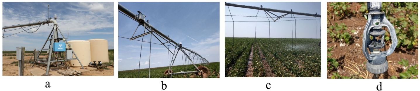
Fig 2. Components of a variable rate irrigation system in a 194-ha farm in Hale County, Texas (a. Control panel, b. Center pivot, c. Variable application of water, and d. Sprinkler head).
