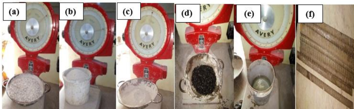
Fig. 1. Materials: (a) gravel, (b) sand, (c) cement, (d) PKS soaked in water for 20mins, (e) water (f) cut GFRP bars
