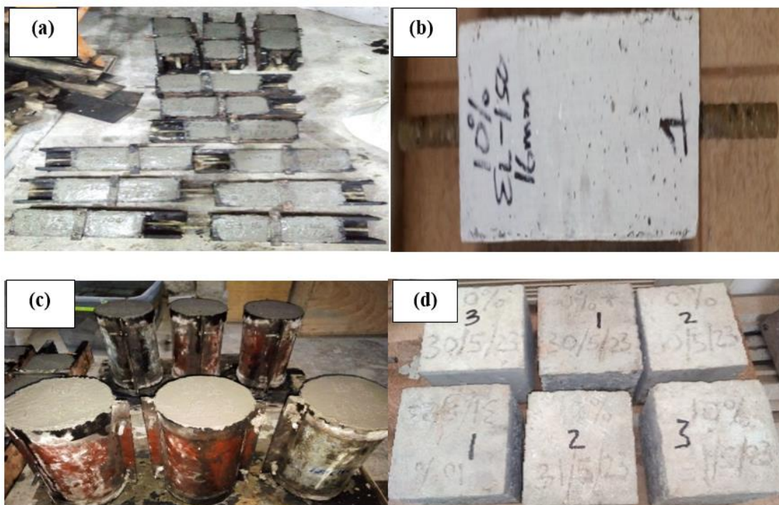
Fig. 3. Specimens: (a) Prism specimens, (b) Hardened prism specimen, (c) cylindrical specimens, (d) cube specimens
