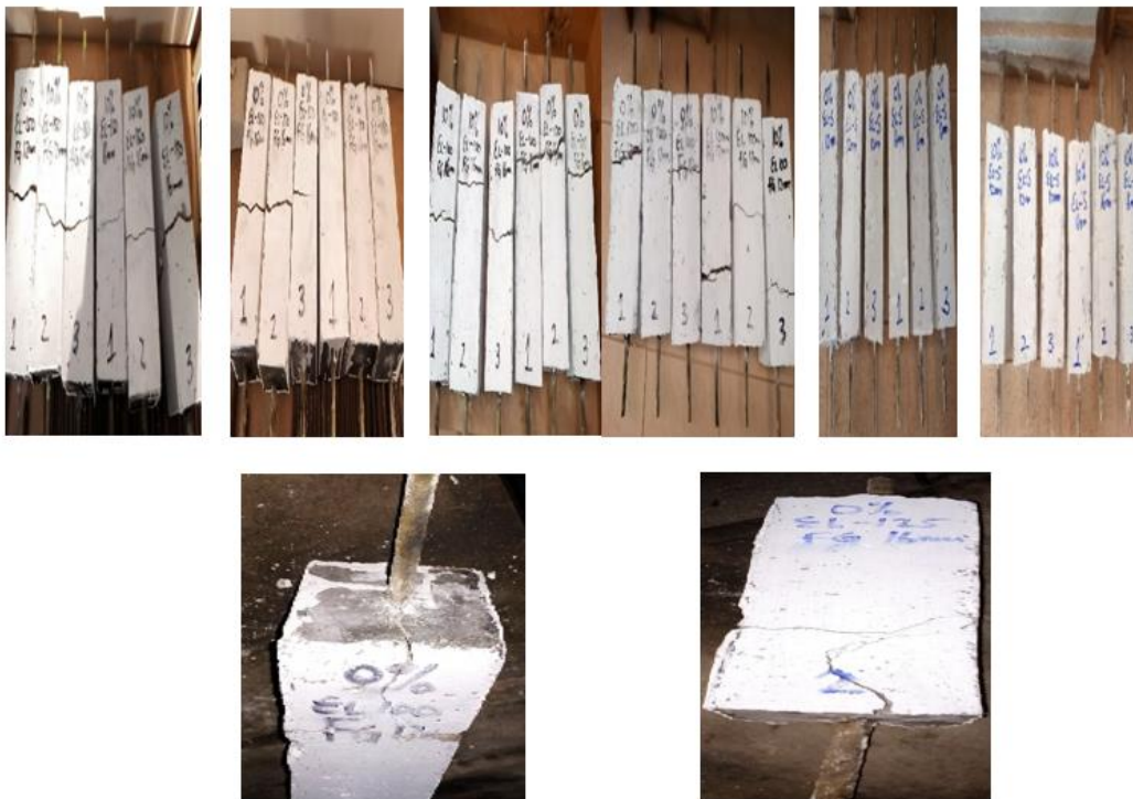
Fig. 10. Tested double pull-out prism specimens with GFRP rebars
