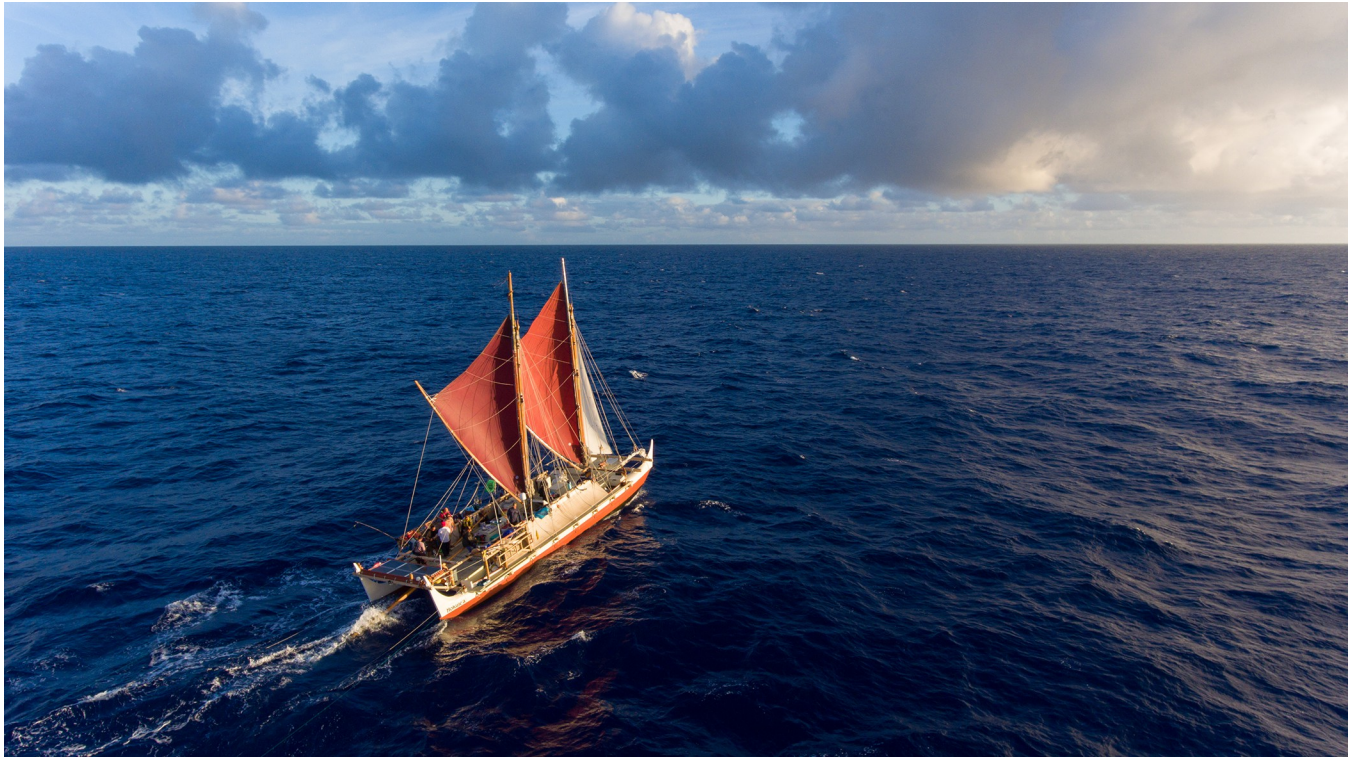
Fig 1. Photograph of Hōkūleʻa under traditional crab-claw sails during a deep-sea portion of the Polynesian Voyaging Society’s 2014–2017 Worldwide Voyage (WWV). Hōkūleʻa is 62 feet (18.9 m) long and 23 feet (7.01 m) wide, with 300 square feet (27.87 square meters) of deck space for an average crew of 12 people. All food and water is stored in the hulls, where crew also sleep—head to toe—under the tan canvas covers. The total covered sleeping area is approximately 138 square feet (12.82 square meters). Solar panels power safety lights and communications. Location information is held in the heads of traditional, non-instrument navigators. Crew fish during daylight hours, cook on a 2-burner propane stove, and wash (people, dishes and clothes) with ocean water. Hōkūleʻa has no engines, refrigeration, nails or screws. Approximately 5 miles (8.05 km) of rope lash her together, and at least 2 miles (3.22 km) of line make up her rigging. A traditional voyaging canoe, she is powered by the wind and steered with large paddles. Copyrighted photo courtesy of Naʻalehu Anthony.
