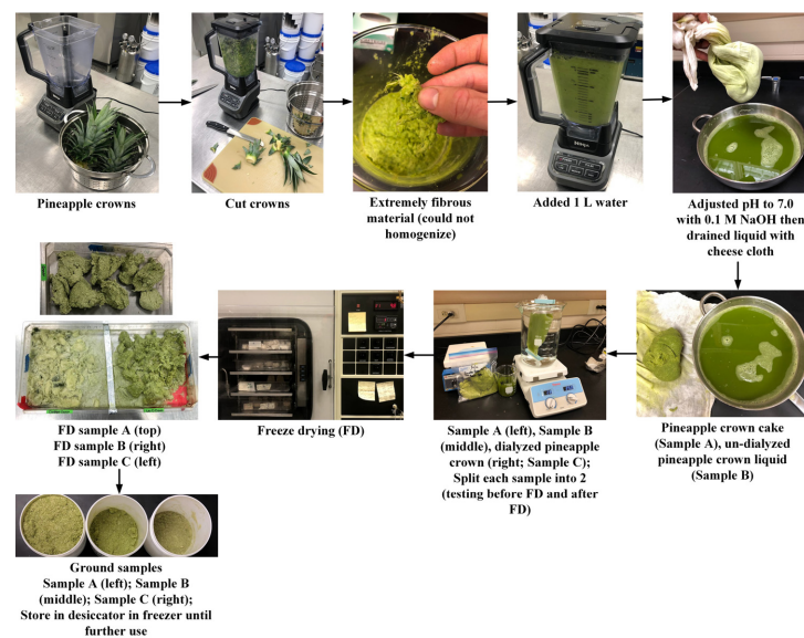
Figure 3. Production of freeze-dried (FD) bromelain powders from pineapple crowns.
