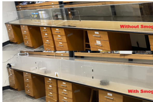
Figure 3. The 5 m chamber with and without smog.
