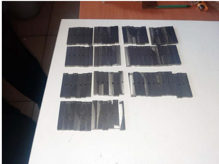
Figure 1. Construction steel specimens prepared for impact toughness testing.
