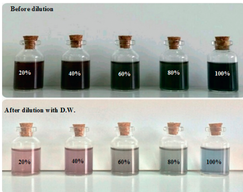
FIGURE 1: The pictures show the color changes after the process of reduction of \text{HAuCl}_4 solution to GNPs using different concentrations of lemon peel extract before and after dilution with distilled water.
