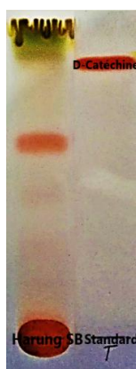
Fig. 5. TLC chromatogram of methanolic extracts of Harungana madagascariensis with D-catechin as standard; developed with Ethyl acetate/Formic acid/Water (100:10:40; v/v/v) and visualized with phosphoric vanillin. Anthocyanins give pink colorings.
