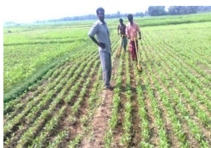
Photo 2. Agricultural Weeder with Nail Assembly having single front wheel and addition of conical rotors and boat for operation in transplanted rice (from left)
