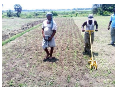
Photo 2. Agricultural Weeder with Nail Assembly having single front wheel and addition of conical rotors and boat for operation in transplanted rice (from left)
