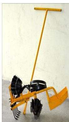
Photo 2. Agricultural Weeder with Nail Assembly having single front wheel and addition of conical rotors and boat for operation in transplanted rice (from left)
