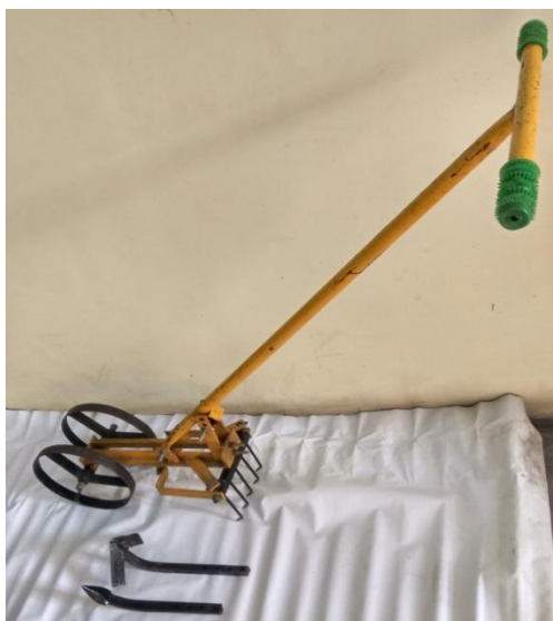
Photo 1. Agricultural weeder with nail assembly, Design registration no. 289754 in class 15-03, dt. 13-09-2019, Patent Office Kolkata, Govt. of India
