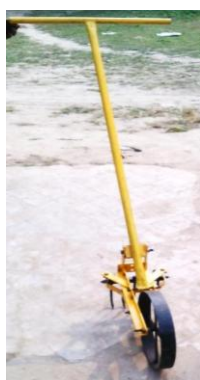
Photo 2. Agricultural Weeder with Nail Assembly having single front wheel and addition of conical rotors and boat for operation in transplanted rice (from left)
