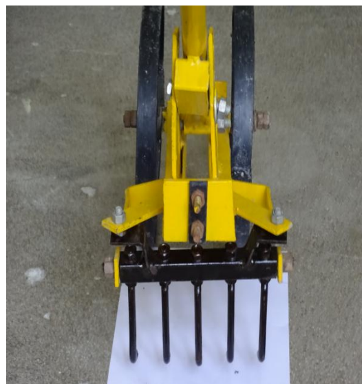
Photo 1. Agricultural weeder with nail assembly, Design registration no. 289754 in class 15-03, dt. 13-09-2019, Patent Office Kolkata, Govt. of India
