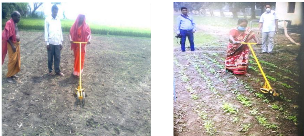
Photo 7. Women working with Agricultural Weeder with Nail assembly in jute and mustard
