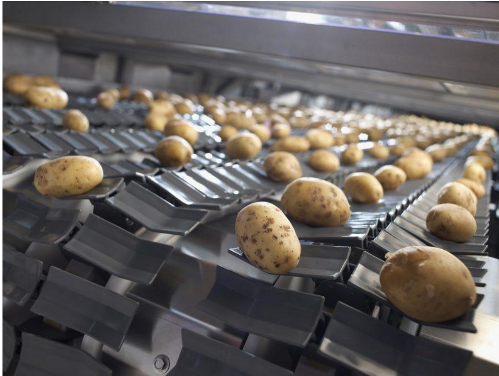
Fig. 2. Sorting potato with an optical sorting machine [7]
