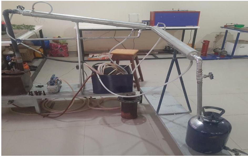
Fig. 2. Locally fabricated pyrolyzer
