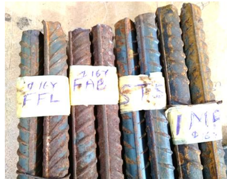
Fig. 1. Typical samples of reinforcing steel bars in Ghana
