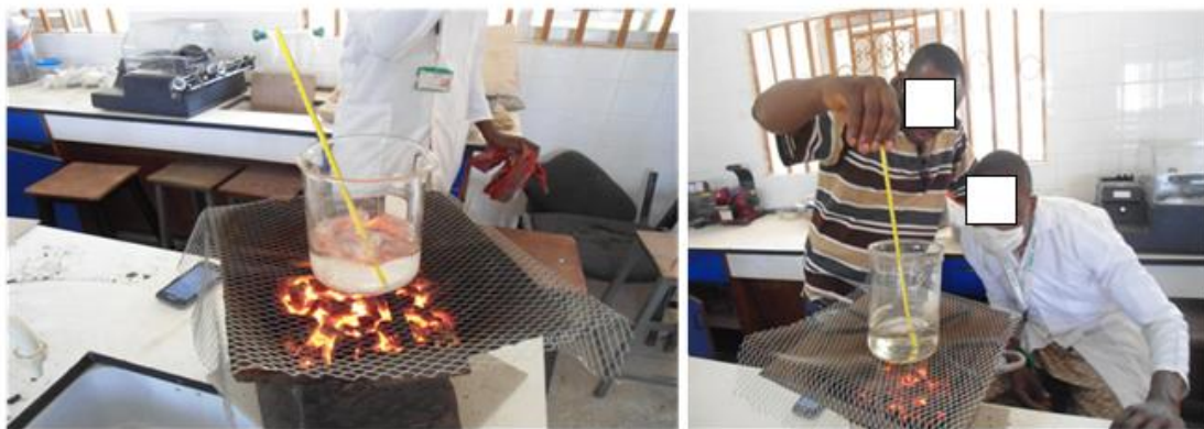
Fig. 8. Combustibility studies for the determination of the coal energy efficiencies and coal combustion pathways by measuring the time it takes same quantity of each of the coal deposits to bring same volume of water to boiling point as well as the temperature achieved at every 2 minutes using local cooking stove
