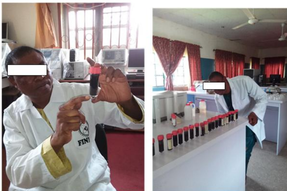
Fig. 11. Defusination experiment involved digestion of the pulverized coals with different types of organic acid and kept to react for 48 hours.
