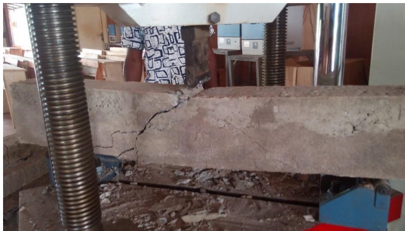
Plate 1. Mode of failure of control beam TI
