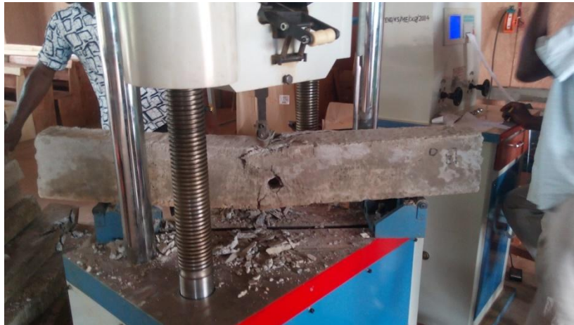
Plate 5. Mode of failure of experimental beam TV
