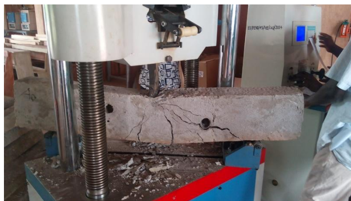
Plate 4. Mode of failure of experimental beam TIV
