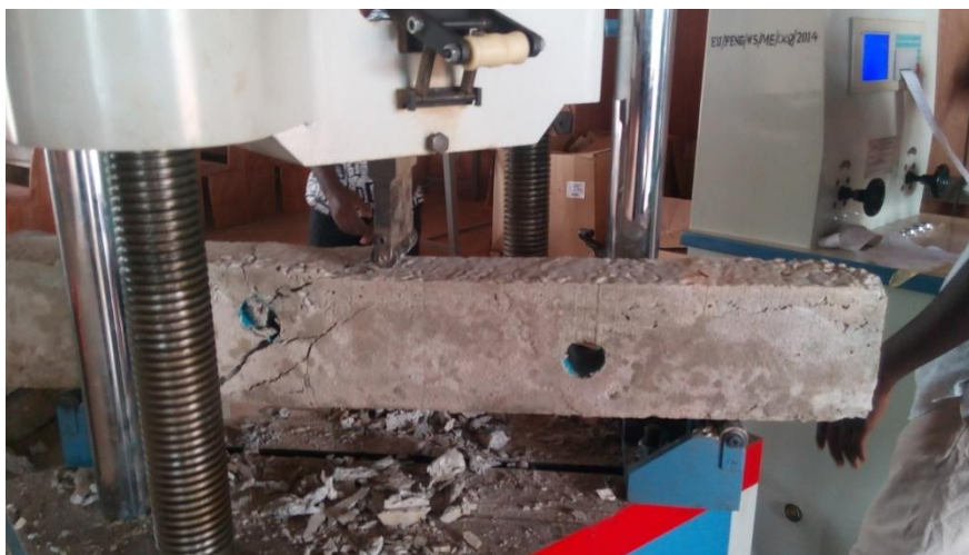
Plate 2. Mode of failure of experimental beam TII
