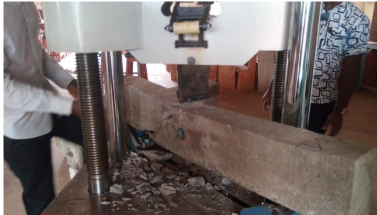
Plate 3. Mode of failure of experimental beam TIII
