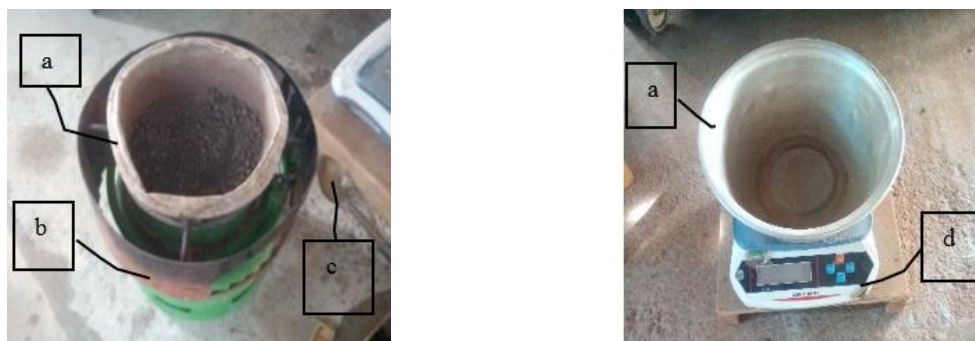
Caption: a : Material bin; b : Gas burner; c : Ladle; d : Scale of 24kg±0,2g Fig. 6. Equipment for water content measuring test
