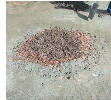
(d) Coarse aggregate and shells of palm kernel added to the mixture of cement, recycled glass powder and fine aggregate
