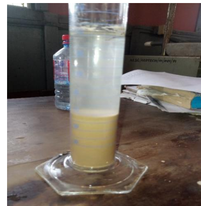
(c) Cylinder allowed to stand for 2 hours
