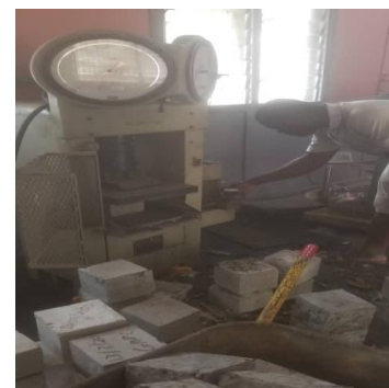
(c) Load applied gradually to the cube
