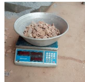
(c) Weighing of coarse aggregate
