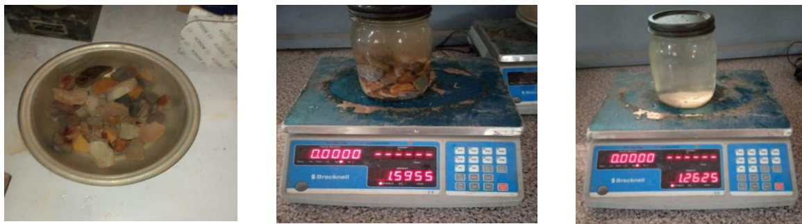
Fig. 6. Determination of water absorption and specific gravity of coarse aggregate
