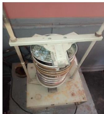
(a) Fine aggregate and sieves mounted on mechanical shaker Coarse aggregate and sieves mounted on shaker
