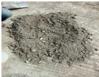
(e) Mixture of fine aggregate, cement, recycled glass powder, coarse aggregate and shells of palm kernel
