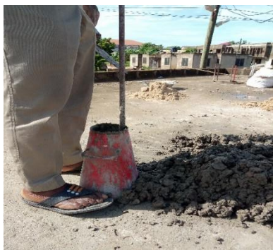
(a) Compacting of concrete sample in slump mold
