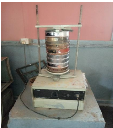
(a) Fine aggregate and sieves mounted on mechanical shaker
