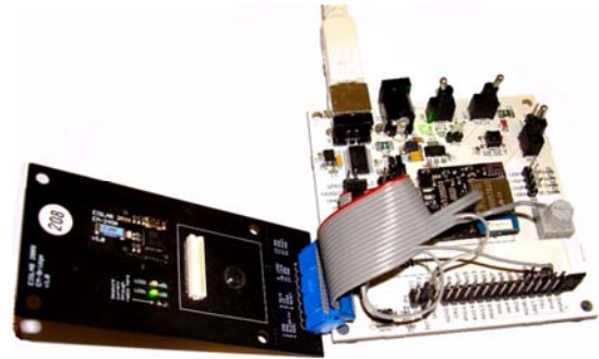
Figure 1. Resource-constrained gateway node, prototype version.
