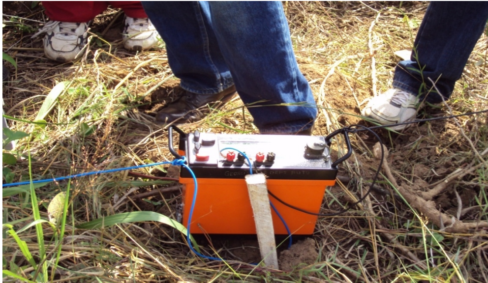
Fig. 4. The versatile ABEM SAS 4000 – High resolution resistivity meter. Positioned at probe point.
