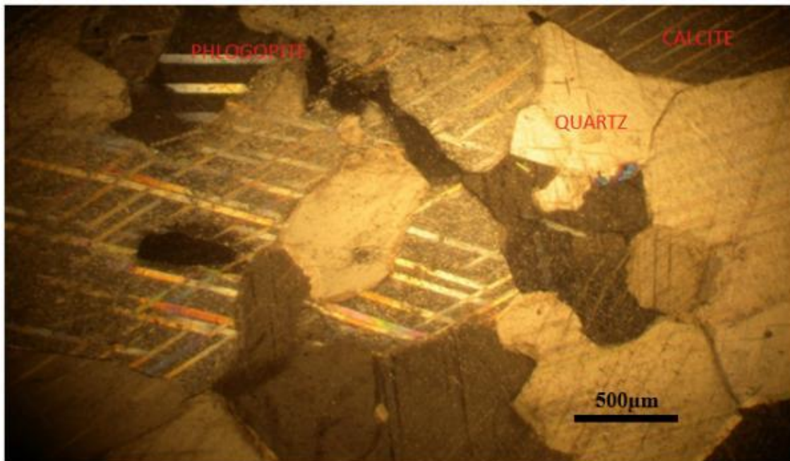
Fig. 2. Photomicrograph of the marble in transmitted light showing: Quartz, calcite, and phlogopite
