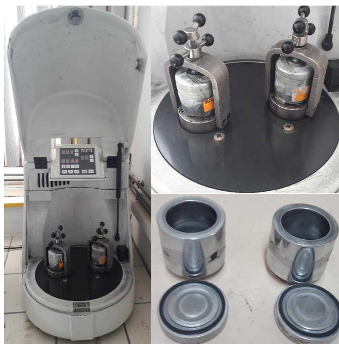
Figure 1. P7 planetary ball mill and milling media used in the experiments.
