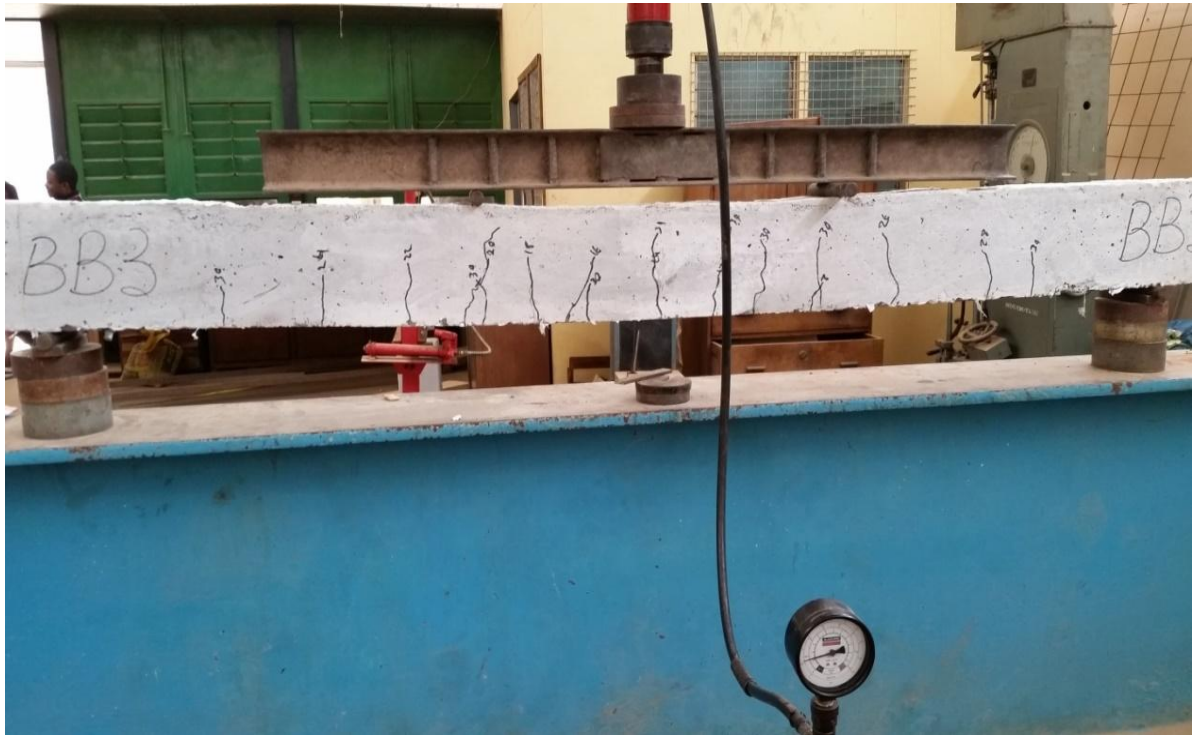
Fig. 5. Crack propagation and characteristics of the 0.25% fibre concrete
