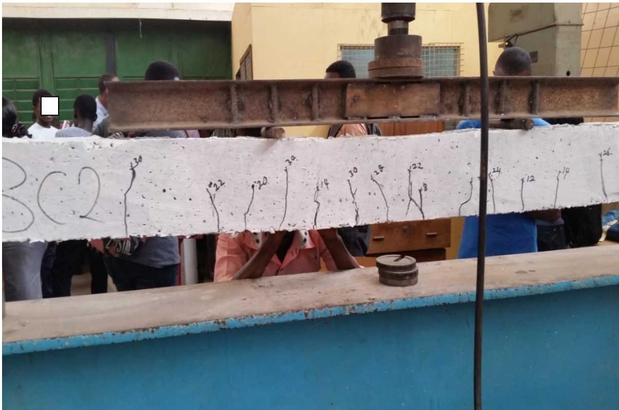
Fig. 6. Crack propagation and characteristics of the 0.5% fibre concrete
