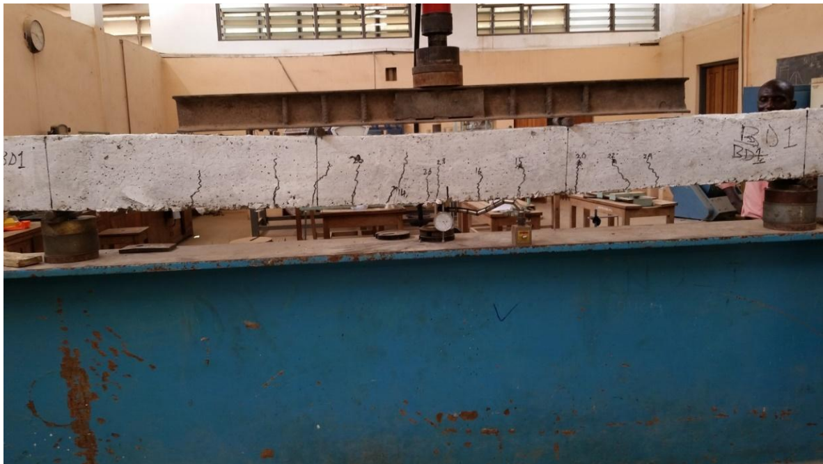
Fig. 7. Crack propagation and characteristics of the 1.0% fibre concrete
