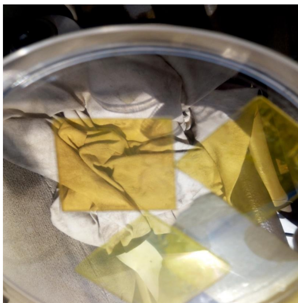
Plate 1. Optical study of CdS samples deposited at 30minutes and 60minutes
