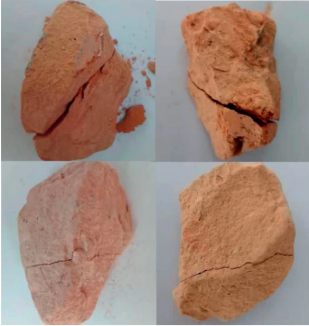
FIGURE 4: Crushing mode of recycled brick particles.
